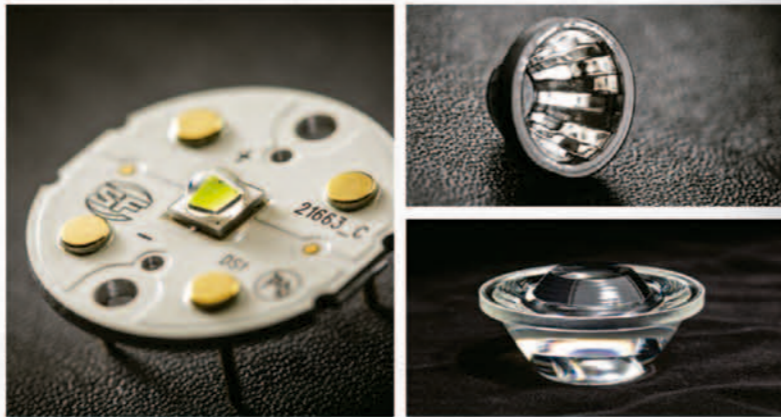
The light from an LED (left) is shaped and formed by one of two precision optics: a reflector (above right) or a TIR lens (below right).
